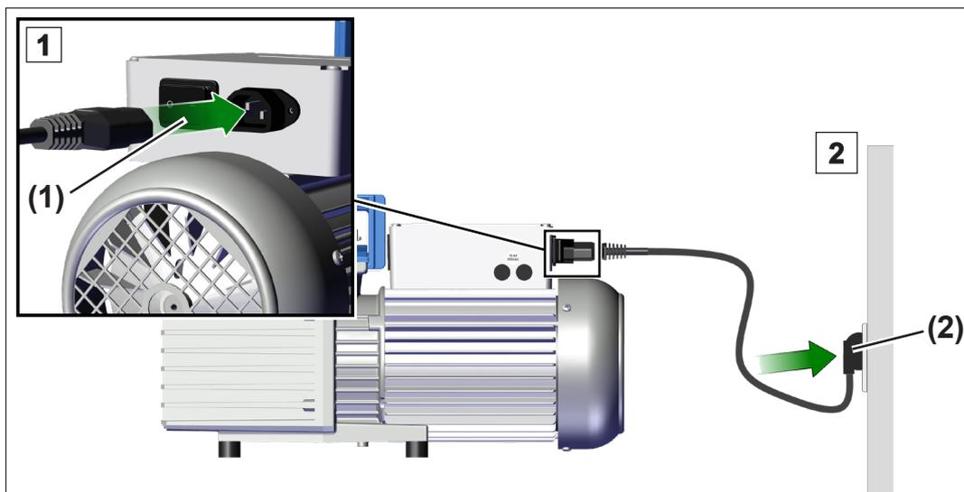
1. Plug connector **(1)** of the power cord into the power connection of the vacuum pump.
