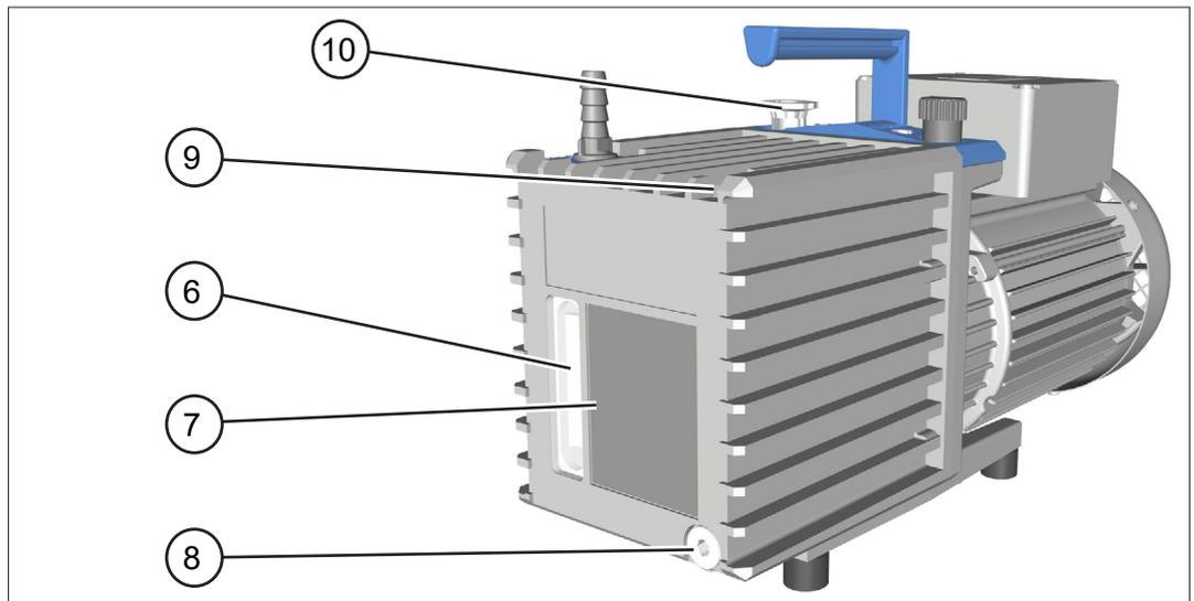
5. Place a suitable receptacle beneath the oil outlet (8). In case, use a funnel.
